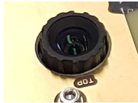
Fig. 12 An example of the satellite wall aperture with piCAM optics and 1 mm thermal gap.
