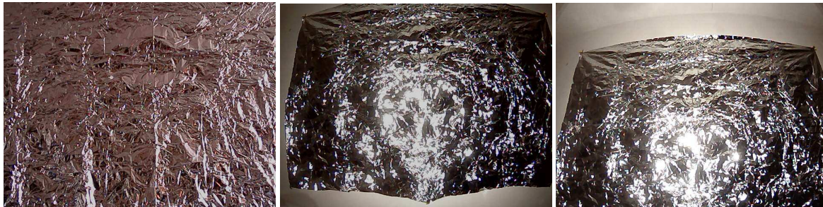
Fig. 8 Example of Aluminum-coated foil with rapid moiré changing patterns. Daylight conditions (left), night/darkness conditions (middle and right) with Evaluation Kit LED Flashlight activated. Foil size 3×2 m, 1 m distance.
