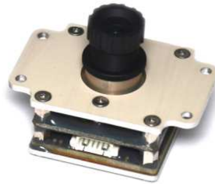
Fig. 1 Digital CubeSat Camera piCAM, Flight Model.
