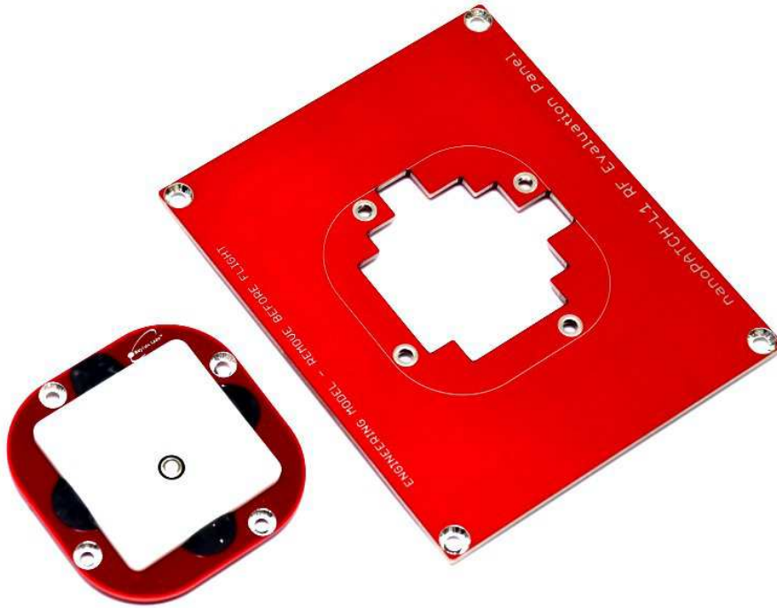
Fig. 4 Engineering Model of the nanoPATCH-L1 unit with red Remove Before Flight finish.
