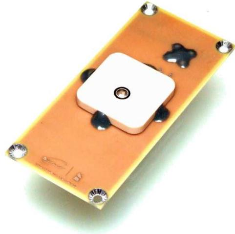
Fig. 1 Micro GPS-L1 Patch Antenna - Flight Model.
